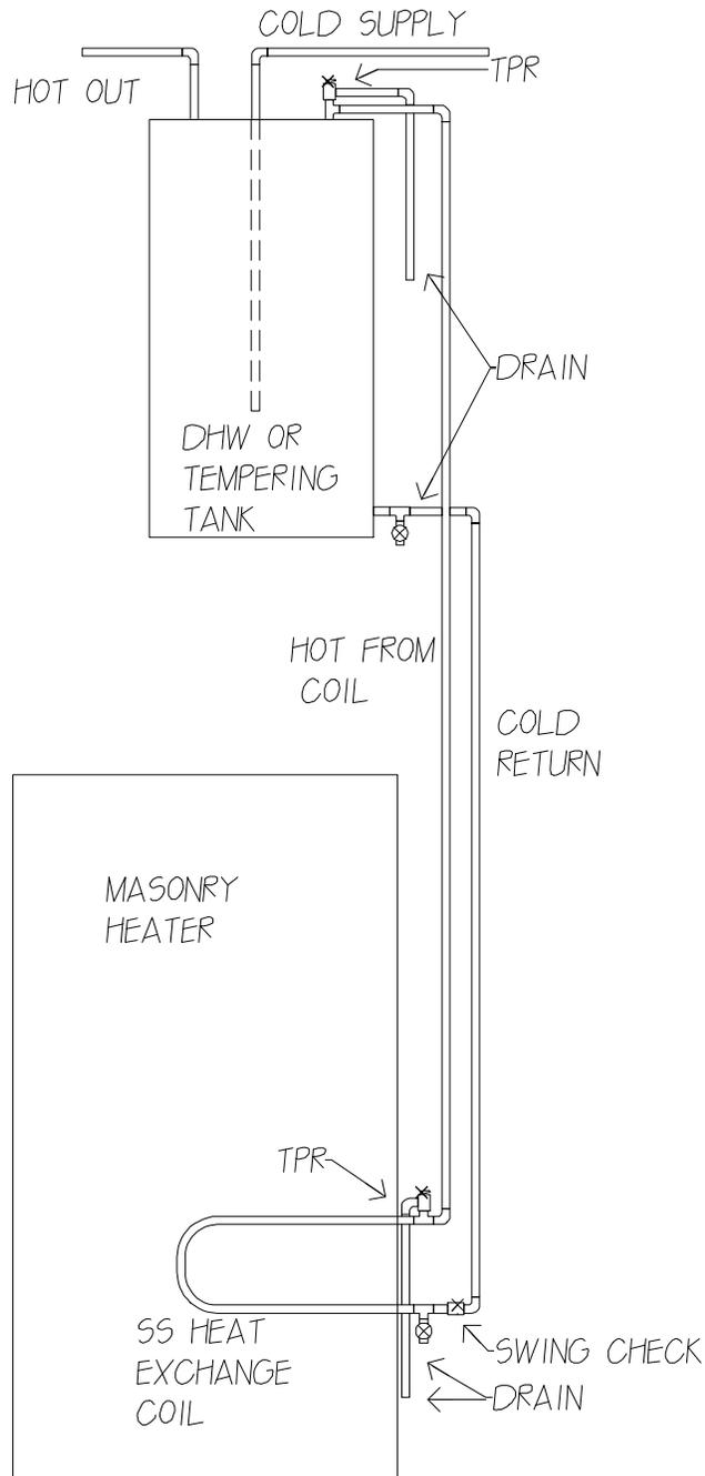
This method allows the most flexibility in locating the tank(s) and provides the greatest amount of heat transfer.
